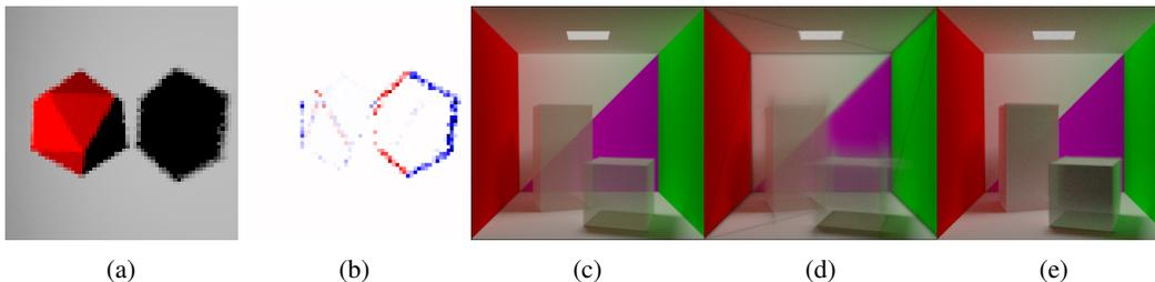
Figure 1: 1b shows the gradients calculated for the icosahedron in 1a for a horizontal translation. 1c shows Cornell box scene with global illumination and Russian roulette termination. 1d has larger  $\sigma$ , resulting in more blur. 1e has smaller  $\gamma$ , resulting in less transparency.
