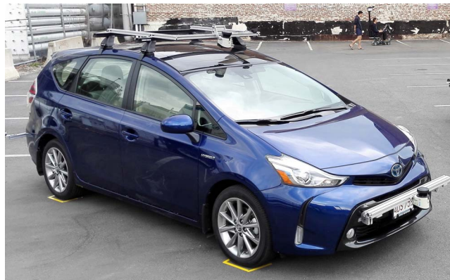
Fig. 1. The converted Toyota 2015 Prius V, a parallel autonomy research platform. The car is outfitted with sensors to enable fully autonomous driving, a drive-by-wire conversion and low-level controllers which are designed to fuse the desired input from the human with the autonomy software control output to provide safe acceleration and speed.
