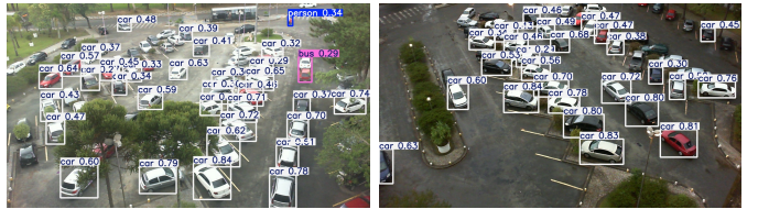
Fig. 5: YOLOv11 applied to UFPR04 (left) and UFPR05 (right).
